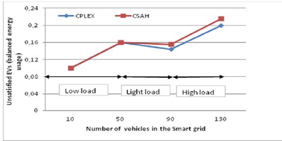
Fig.6. Performance of both CPLEX and heuristic based on balanced energy usage on EVSEs
