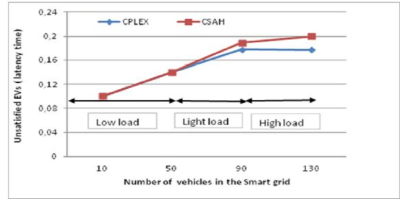
Fig.5. Performance of both CPLEX and heuristic based on latency time on EVs
