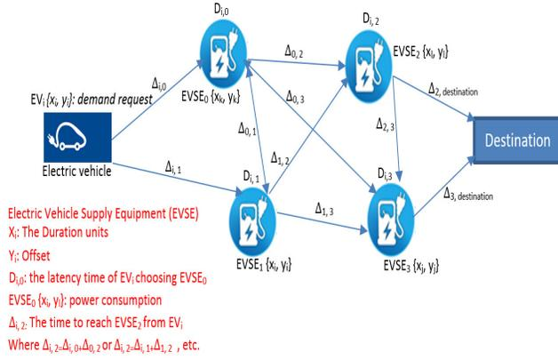
Fig.2. Connectivity graph: An example network of different paths connecting EV<sub>i</sub> to a destination.
