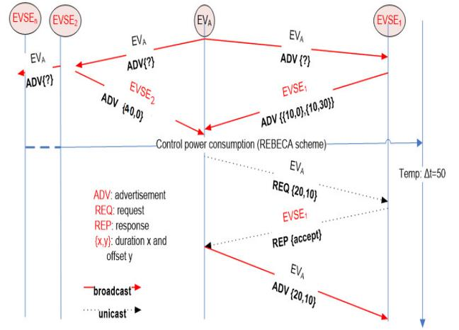
Fig.4. Sequence diagram of power discovery messages between EVs and EVSEs based on the example in Fig. 3.
