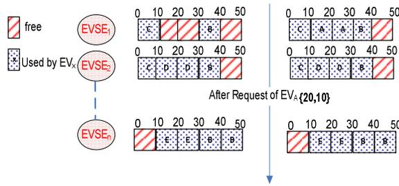
Fig.3. An example of dynamic adjustment of electricity use on EVSEs using random access allocation algorithm
