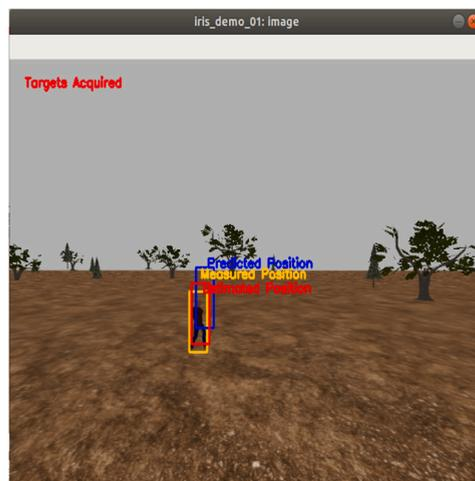
Fig. 8. UAV camera capture when detecting the target.
