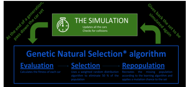
Fig. 3: The process of simulating consists of three phases: (1) the evaluation, (2) the selection and (3) the repopulation.
