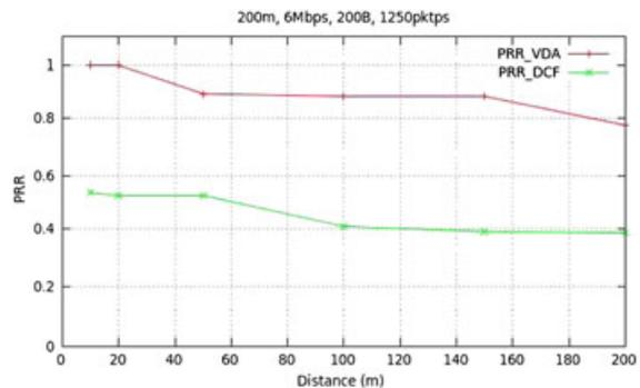
**Figure 9.** The reception probability of both Vehicular Deterministic Access (VDA) and Distributed Coordination Function (DCF) while varying the distance – *range: 200 m, message frequency: 1250/s; data rate: 6 Mbps; message size: 200 bytes.* PRR, packet reception rate.
