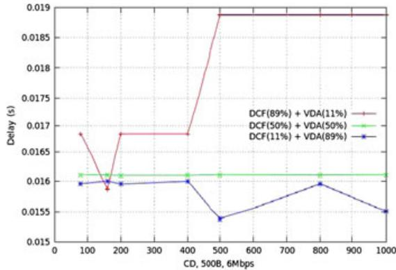
**Figure 13.** 802.11p/VDA delay without EVDA improvement. VDA, Vehicular Deterministic Access; DCF, Distributed Coordination Function; EVDA, extended VDA; CD, communication density.
