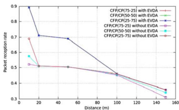
**Figure 16.** Reception probability for Distributed Coordination Function Vehicles with and without Extended Vehicular Deterministic Access (EVDA). CFP, contention free period; CP, contention period.
