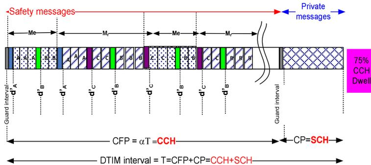
**Figure 4.** Vehicular Deterministic Access opportunity schedule for emergency ( $M_e$ ) and routine ( $M_r$ ) messages in an example of extended Vehicular Deterministic Access (75% contention free period/contention period (CFP/CP) dwell time ratio) for vehicles A, B, and C with Vehicular Deterministic Access option. CCH, control channel; SCH, service channel; DTIM, delivery traffic indication message.
