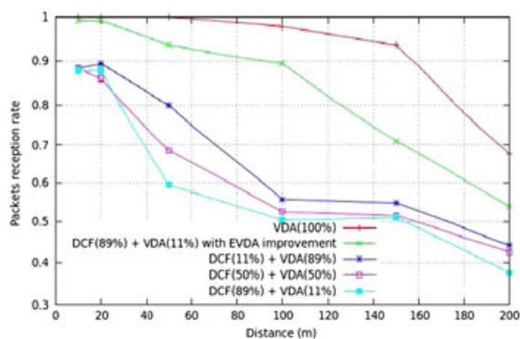
**Figure 14.** 802.11p/VDA reception probability with and without EVDA improvement. VDA, Vehicular Deterministic Access; DCF, Distributed Coordination Function; EVDA, extended VDA.
