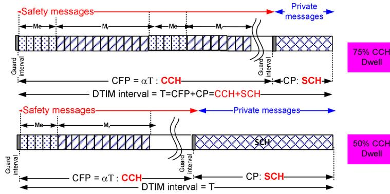
**Figure 1.** Vehicular Deterministic Access opportunity schedule for emergency ( $M_e$ ) and routine ( $M_r$ ) messages in Vehicular Deterministic Access. CFP, contention free period; CCH, control channel; CP, contention period; SCH, service channel; DTIM, delivery traffic indication message.
