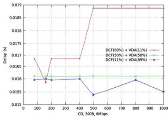
**Figure 13.** 802.11p/VDA delay without EVDA improvement. VDA, Vehicular Deterministic Access; DCF, Distributed Coordination Function; EVDA, extended VDA; CD, communication density.
