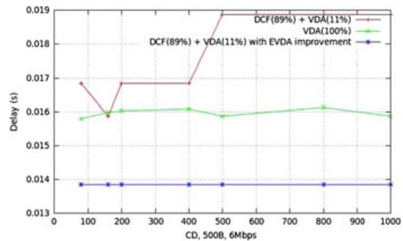
**Figure 12.** 802.11p/VDA delay with and without EVDA improvement. VDA, Vehicular Deterministic Access; DCF, Distributed Coordination Function; EVDA, extended VDA; CD, communication density.
