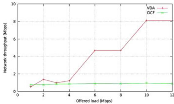
**Figure 10.** The network throughput of both Vehicular Deterministic Access (VDA) and Distributed Coordination Function (DCF).
