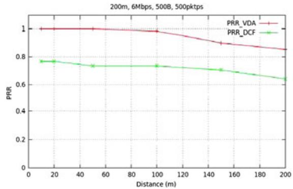
**Figure 8.** The reception probability of both Vehicular Deterministic Access (VDA) and Distributed Coordination Function (DCF) while varying the distance – *range: 200 m; message frequency: 500 packets/s; data rate: 6 Mbps; size message: 500 bytes.* PRR, packet reception rate.
