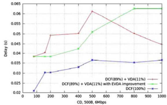
**Figure 11.** 802.11p/DCF delay with and without EVDA improvement. VDA, Vehicular Deterministic Access; DCF, Distributed Coordination Function; EVDA, extended VDA; CD, communication density.
