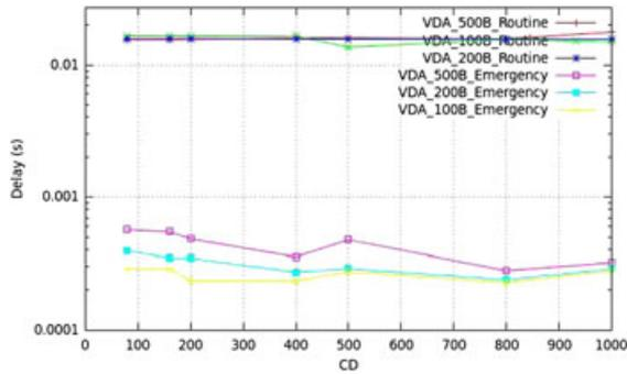
**Figure 6.** The delay of both emergency and routine messages in Vehicular Deterministic Access (VDA) scheme while varying communication density and packet size.
