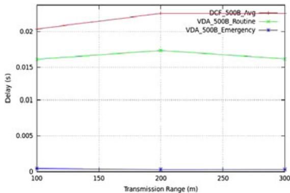
**Figure 7.** The delay of both emergency and routine messages in Vehicular Deterministic Access (VDA) scheme compared with Distributed Coordination Function (DCF) scheme: *messages frequency: 25 messages/s; vehicle density: 10–100 vehicle/km/lane; data rate: 6 Mbps; message size: 500 bytes.*
