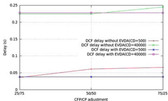
**Figure 15.** Delay for Distributed Coordination Function (DCF) vehicles with and without Extended Vehicular Deterministic Access (EVDA). CD, communication density; CFP, contention free period; CP, contention period.
