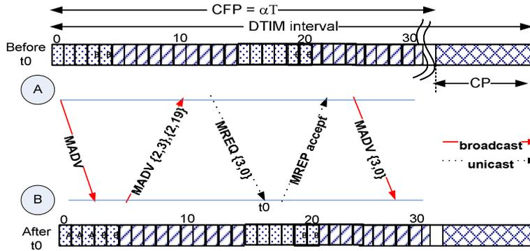
**Figure 2.** Example of the negotiation of an Mesh Coordinated Channel Access opportunity (MCCAOP) from node A to node B. Notation  $x, y$  means that the MCCAOP has duration  $x$  and offset  $y$  [5]. CFP, contention free period; CP, contention period; DTIM, delivery traffic indication message.
