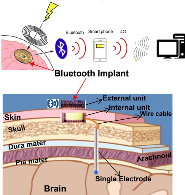
Fig. 4. Novel Implant Design using a Bluetooth connection with the cellphone along with a TCP/IP connection with the server.
